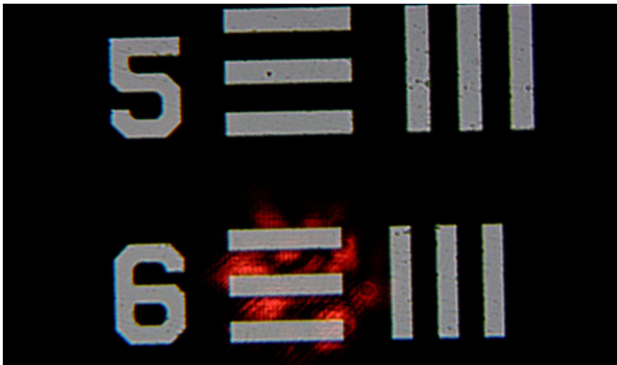
USAF 1951 Chart (Group 5, Element 6 - 8.77 microns line spacing), 20X objective
